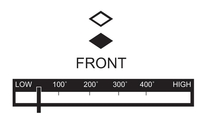
slider replaces knob and shows both range of heat and approximate temperature
