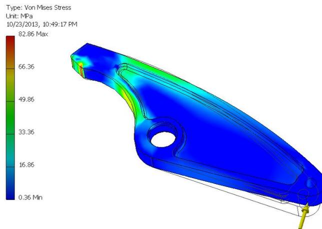
17. After reviewing the results you will notice a high stress area near the clamping surface. Review the convergence by clicking **Result panel | Convergence** to open the **Convergence Plot** dialog. You will see the simulation as not converged yet with a rate of 26.25%. We will cover this in greater detail later.
