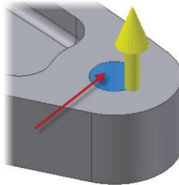
13. In the **Bearing Loads** dialog enter the following directional information that was direction from an assembly motion analysis:
