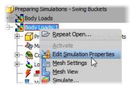
5. In the **Simulation Properties** dialog, enter **Body and Force Loads** in the **Name** field. Click **OK** to dismiss the dialog.
