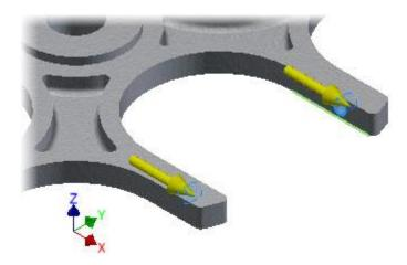
9. Enter 1600N for the Magnitude and click Apply, but do not dismiss the Bearing Load dialog.
