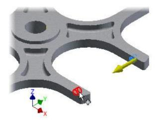
8. Pick the **Direction** button from the **Bearing Load** dialog. Select an **edge** that is aligned with the **positive X** axis so that the forces point in the positive X direction, outward from the center of the model. Use the **Flip Direction** button if necessary.
