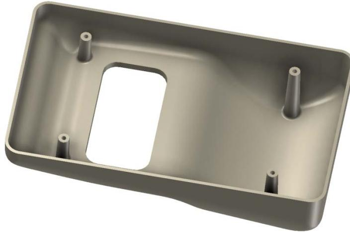
7: As described in the previous projects a standard feature on plastic parts is seam where two cases meet. Let's use the lip tool again to create a lip feature around the upper case.
