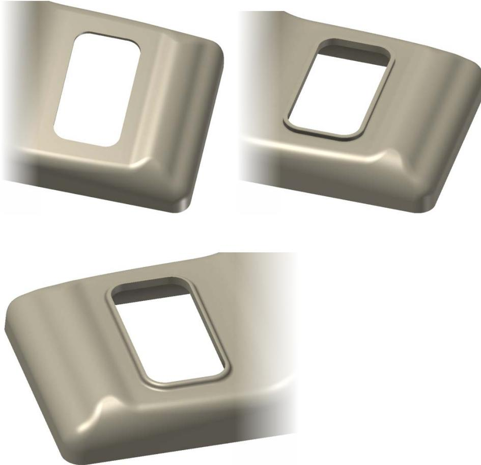
5: In order for plastic parts to be molded it is necessary for plastic parts to have surfaces that are slightly angles. These angles surfaces are commonly called **Draft** angles and allow for a plastic part to be removed from its mold. Let's create a draft angle on the display opening.
