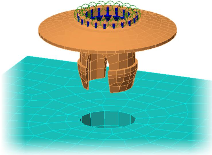
15. Setup a **Surface Contact** pair between the surfaces marked below. There should be a total of 16 contact pairs created. Each of the 8 surfaces on the Push Bushing part should be paired with both of the hole surfaces.
