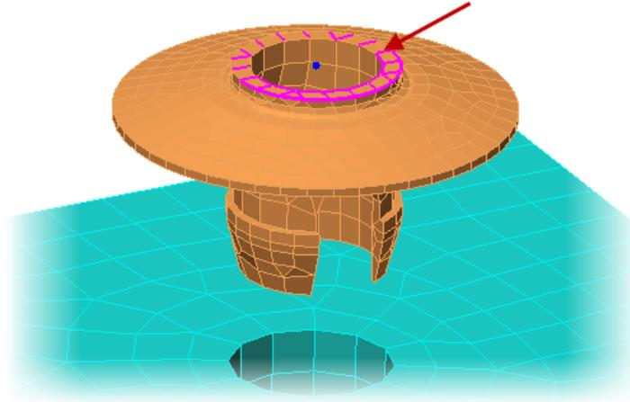
10. Right-Click in the graphics window and select **Add | Surface Boundary Condition**. Check the **Tx** and **Ty** checkboxes to lock the X and Y translational degrees of freedom. Click **OK** to complete. This will help hold the position of the part as it is pressed into the plate.
