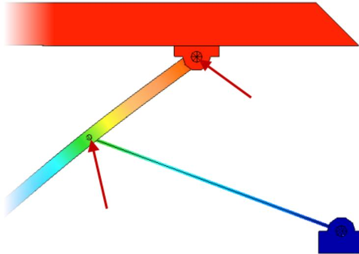
54. Right-Click in the graphics window and select **Graph Value(s)**. This will open a graph showing the displacement of the two nodes over the time of the simulation. You will notice the node where the actuator mounts maintains a nice linear movement. Where the displacement for the node on the top is pulsating.
