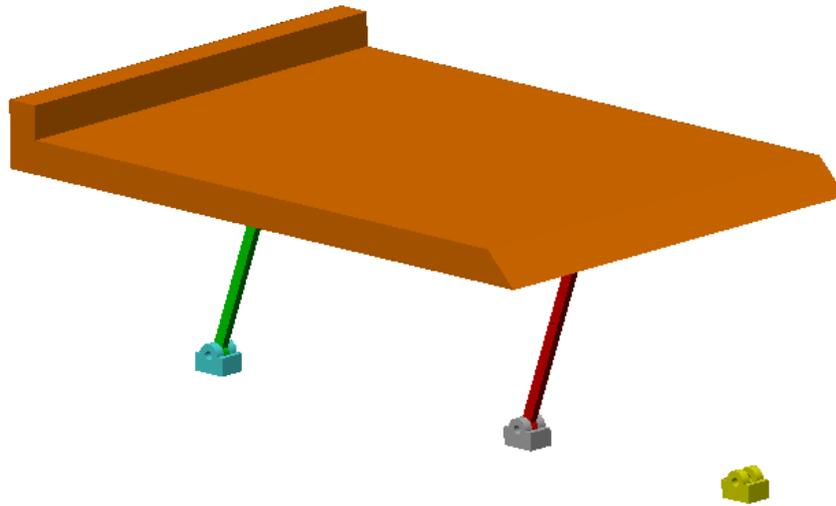
2. Click **Mesh tab | Mesh panel | 3D Mesh Settings**. Within the **Model Mesh Settings** dialog click the **Options** button. Select **Absolute Mesh Size** as the type and enter **0.625** as the **Mesh Size**. Click **OK** to accept the mesh options.
