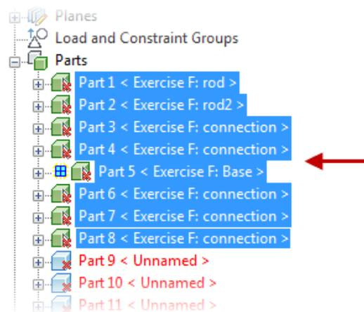
31. Right-Click on one of the selected headings. Select the **Edit | Element Data** option to open the **Element Definition** dialog. Ensure **Large Displacement** is set as the **Analysis Type** and click **OK**.
