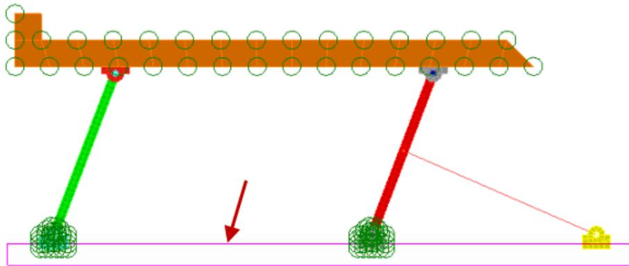
45. To lock the position of the clevis parts click on **Setup tab | Constraints panel | General Constraint** to open the **Bounding Condition** dialog. Click the **Fixed** button to lock all degree of freedom of the surfaces. Click **OK** to complete the assignment.
