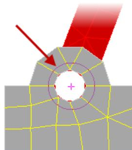
14. Click **Mesh tab | CAD Additions panel | Joint** to open the **Create Joint** dialog. Verify the joint type is **Pin Joint** and click **OK** to create the joint.
