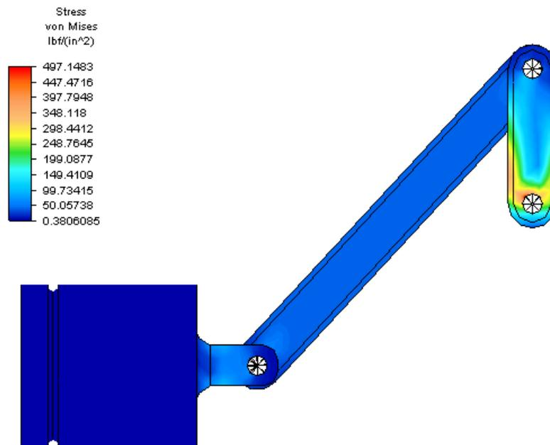
71. Click **Results Inquire** tab | **Probes** panel | **Maximum** to display a probe where the maximum stress is located.
