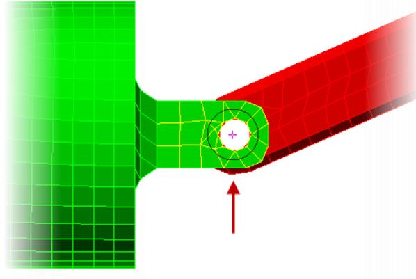
14. Click **Mesh tab | CAD Additions panel | Joint** to start the process of create a joint. The **Create Joint** dialog box is displayed.
