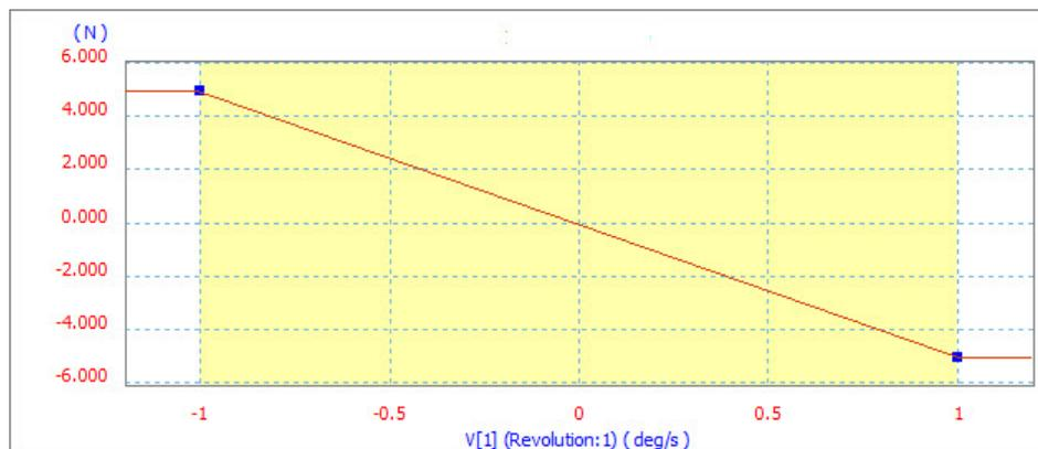
To create a smooth transition in the resistive force, you can change the ramp from a linear ramp to a cubic ramp.
