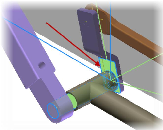
21. To ensure the two coordinate systems are in alignment **Flip Z Direction** on **Component 2**.
