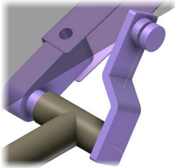
46. Select the circular edge to set the origin of the coordinate system for the second component.
