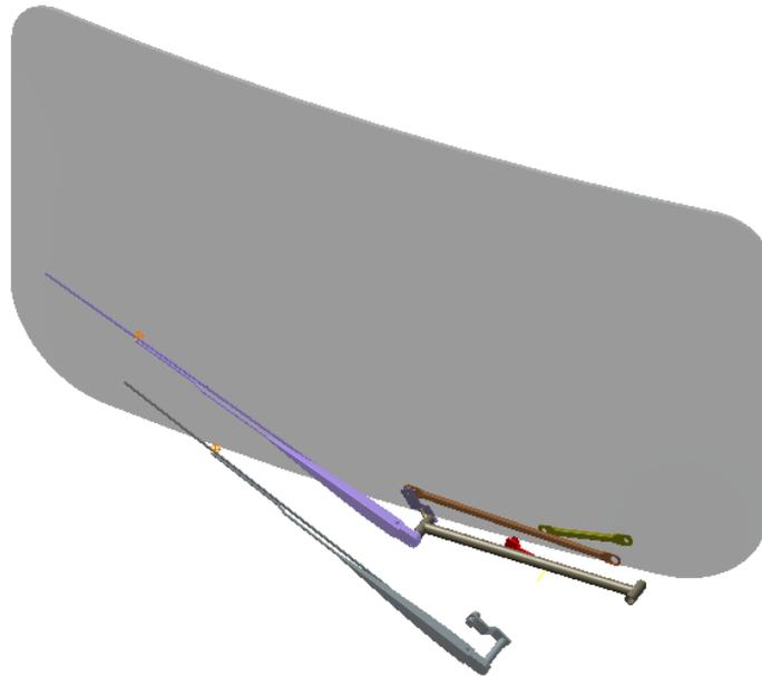
2. **Zoom** in to the wiper assembly as shown. The subassemblies *Brush\_asm\_left* (1) and the *Complete\_wiper\_left\_asm* (2) must move as a unit. In the next steps, you weld the two subassemblies together.
