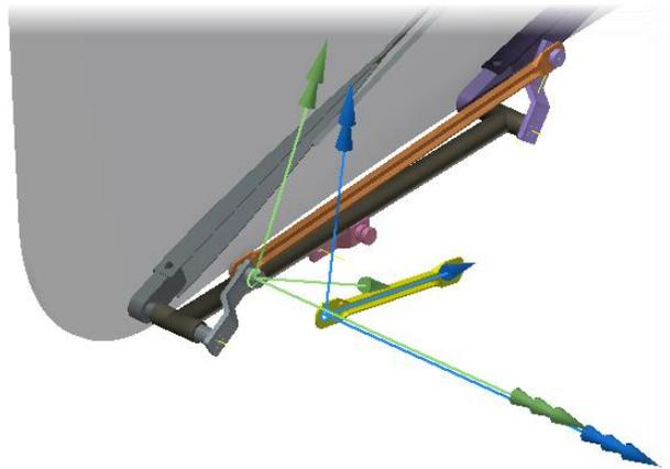
18. Click **Apply**. The *Crank\_motor2* moves to the correct position. The **Insert Joint** dialog box remains open.
