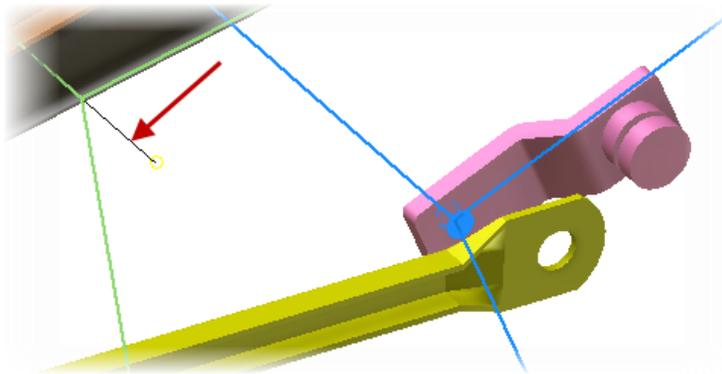
11. Click **OK**. The cylindrical joint enables *the Motor\_Crank\_Asm* to rotate freely around the work axis and move along the work axis.
