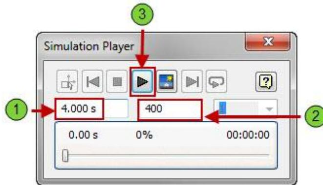
With the simulation set to four seconds the *Motor\_Crank\_Asm* component will make two complete revolutions.
