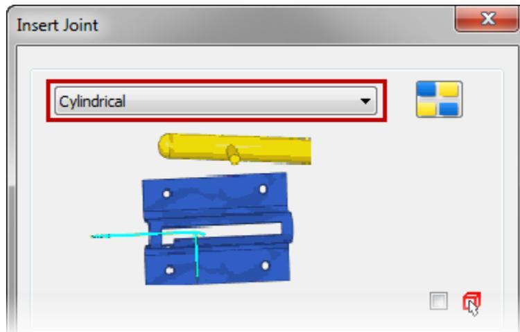
8. For the **Component 1 Z Axis** select the hole of the *Motor\_Crank\_Asm* as shown.
