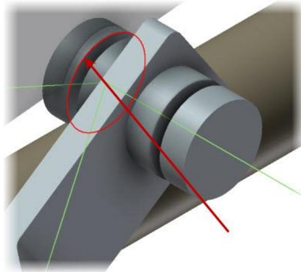
38. Review the orientation of the X axis (1) and the Z axis (2). The Z axes are pointing in the same direction, so the components maintain their current orientation. The X axes are pointing in nearly opposite directions, which will cause the *Inter\_Crank* part to rotate so that its X axis matches the direction of the X axis on the *Complete\_wiper\_left\_asm* subassembly. Next, you reverse the direction of the *Complete\_wiper\_left\_asm* X axis to minimize the rotation.
