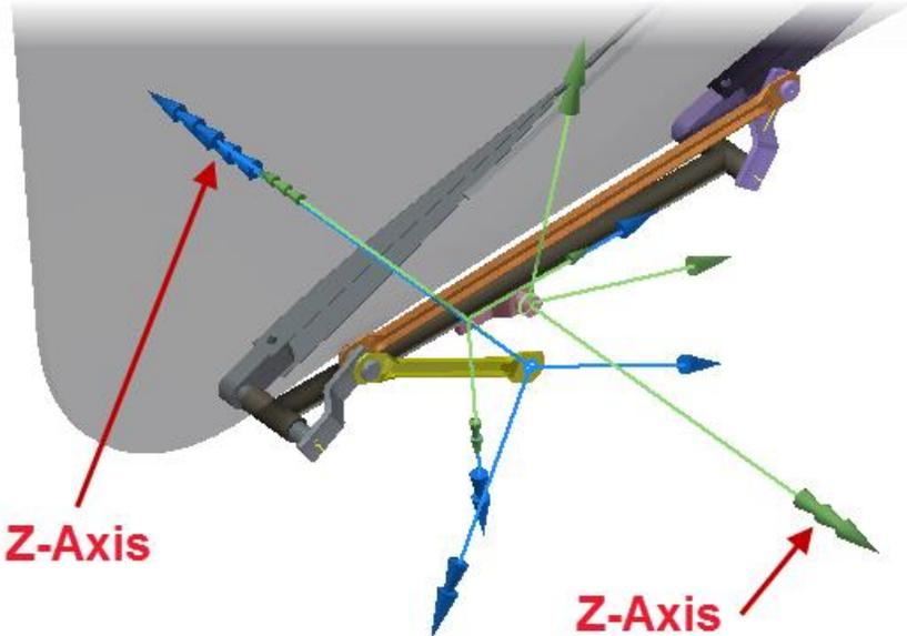
24: Under *Component 2*, click Flip Z Axis Direction as shown to reverse the direction of the Z axis.
