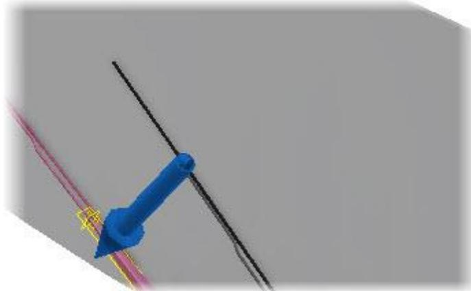
The resistive force maintains the same direction on the wiper throughout the simulation. The resistive force of the wiper should always be opposite to the motion. You use the **Input Grapher** to change the direction of the force when the wiper changes direction.
