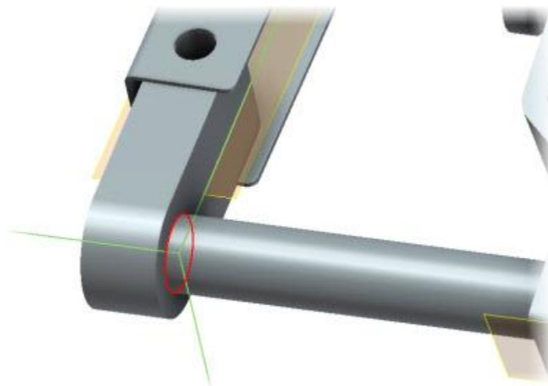
13. Notice that the two coordinate systems are in general alignment. Click **OK** to create the joint. Now notice that the two welded group components moved into position as one single item.
