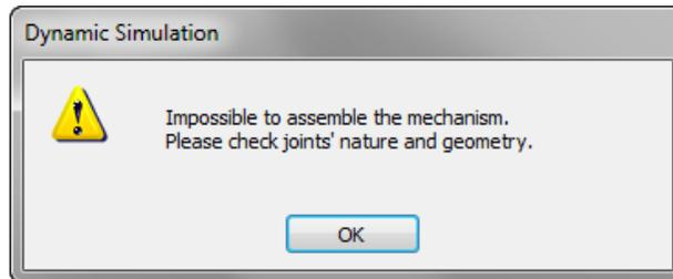
50. In the browser, review the **Standard Joints** group. The *Revolution:4 (Inter\_Crank:1, Complete\_wiper\_right\_asm:1)* joint is shown with an icon indicating that it has been suppressed. Next you will repair this redundancy in the joint of being over constrained.
