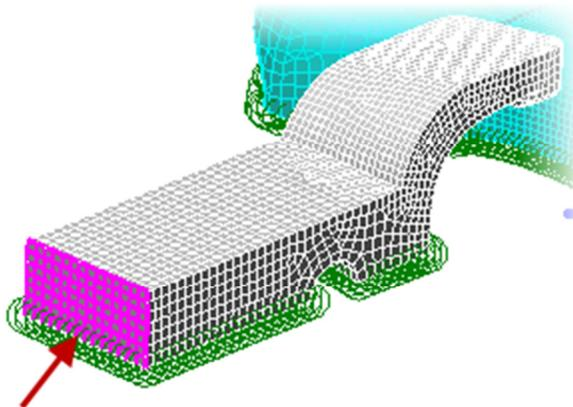
47. Add a **General Constraint** to this surface constraining the **Tz** DOF. This will preview the part from moving in the Z direction.
