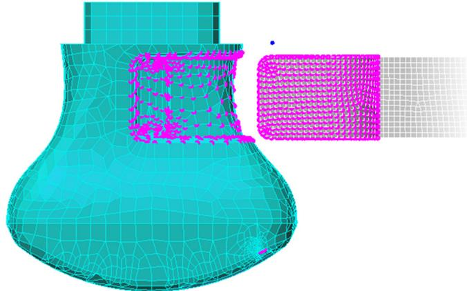
18. To ensure the mesh is controlled in this area we will add mesh refinement points to each of the selected nodes. Click **Mesh tab | Refinement Points panel | Add to Selected Nodes**.
