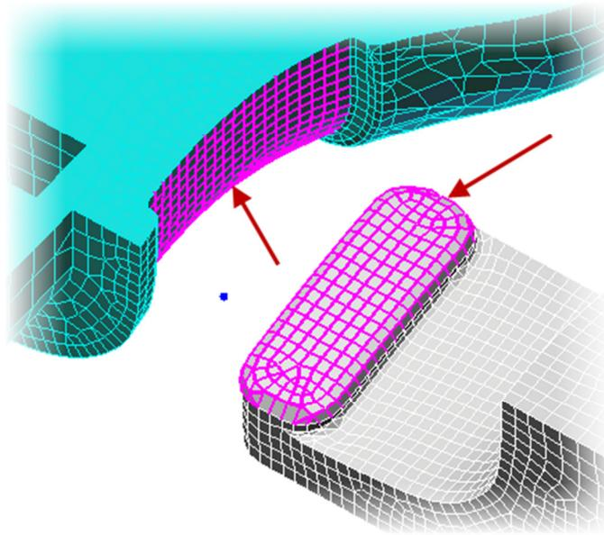
29. To establish a contact relationship between these two surfaces click **Setup tab | Contacts panel | Surface-to-Surface Contact**. Then hit **ENTER** to accept the default contact name in the **FEA Editor browser**. This contact will allow the surfaces to touch each other or separate but not interfere.
