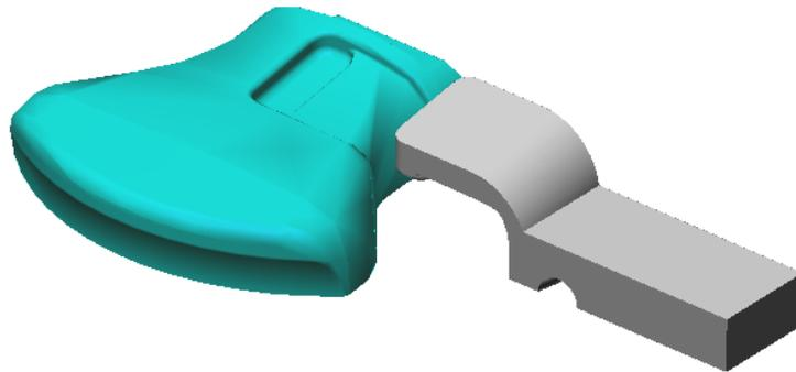
13. Mesh the model using the default setting by clicking **Mesh tab | Mesh panel | Generate 3D Mesh**.
