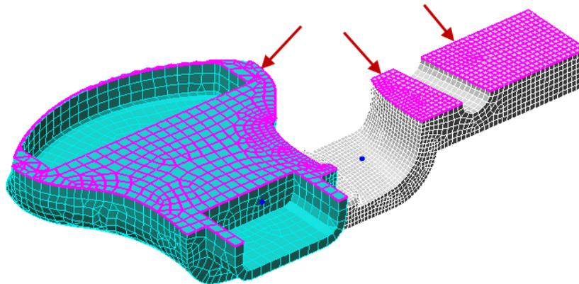
42. With only half of the model imported into Autodesk Simulation we will add a symmetry constraint to the model. Click **Setup tab | Constraints panel | General Constraint**.
