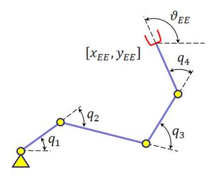
Determine the analytic relationship between a set of joint angles (also called a *configuration*) and the end-effector placement (this relationship is called *direct kinematic*). Write then a computationally efficient MATLAB function  $ps9_1_DK()$  (you will call this function many times ...) that calculates the end-effector *placement* given the manipulator *configuration*:
