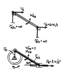
16-126. At a given instant, the gear has the angular motion shown. Determine the accelerations of points A and B on the link and the link's angular acceleration at this instant.
