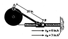
Velocity Analysis: The angular velocity of link AB can be obtained by using the method of instantaneous center of zero velocity. Since  $\mathbf{v}_A$  and  $\mathbf{v}_B$  are parallel,  $r_{AHC} = r_{BHC} = \infty$ . Thus,  $\omega_{AB} = 0$ . Since  $\omega_{AB} = 0$ ,  $\upsilon_A = \upsilon_B = 6$  in./s. Thus, the angular velocity of the wheel is  $\omega_W = \frac{\upsilon_A}{r_{OA}} = \frac{6}{5} = 1.20$  rad/s.
