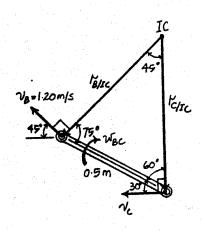
16-97. If rod AB is rotating with an angular velocity  $\omega_{AB} = 3 \text{ rad/s}$ , determine the angular velocity of rod CD at the instant shown.
