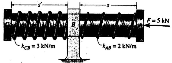
$$F_{CB} = k_{CB}x = 3000x \quad F_{AB} = k_{AB}x = 2000x$$
