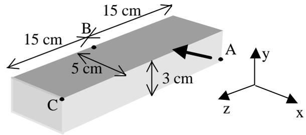
**2. (20 points)** The body shown is subjected to two forces and it is maintained in the position shown by a hand which firmly grips the handle at A. The 25 lb force accounts for the weight. The 10 lb force is applied in the middle of its face. The handle comes out from the middle of its face.
