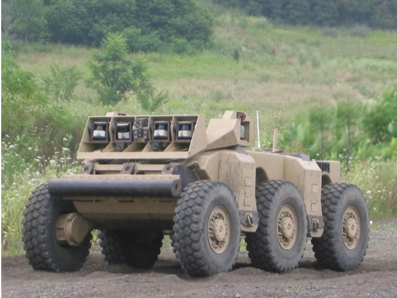
Crusher with sensors
