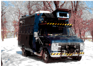
Navlab II: 1990-92 Natural Terrain, 20km/hr Freeway, 70km/hr, 150km Cameras, Laser range finder, Sparc 20s
