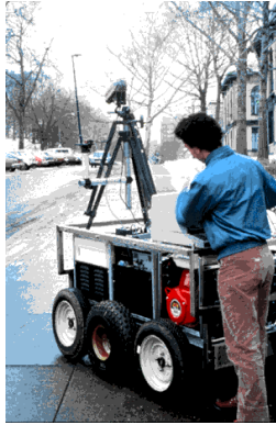
Terregator: ~1985 Campus pathway <100m/hr, 100m total Camera, Off-board computing
