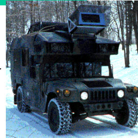
Navlab II: 1990-92 Natural Terrain, 20km/hr Freeway, 70km/hr, 150km Cameras, Laser range finder, Sparc 20s
