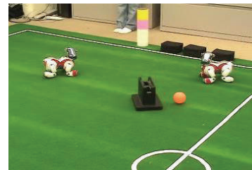
(i) Case (3c): All of the kick hypotheses expire and the robot tracks the teammate's reported hypothesis (the ball is hidden from the first robot's view)
