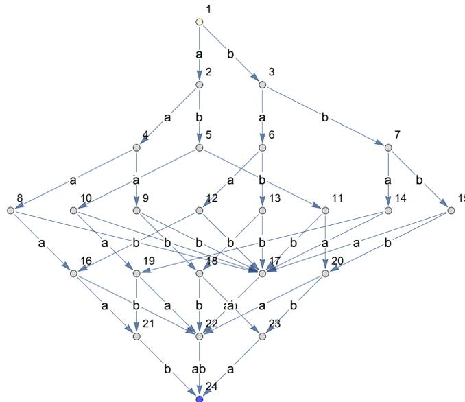
This is the partial DFA without sink, the top state is initial and the bottom state final.
