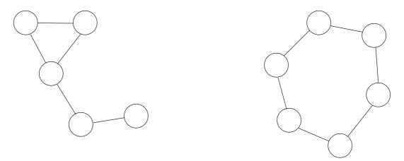
Note that the following are legal frequency assignments to these two tower configurations. However, the second arrangement does not use the fewest number of frequencies possible, since the tower with frequency 5 could have frequency 1.
