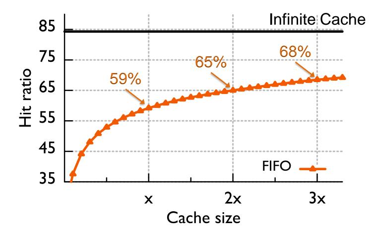
• "Infinite" size ratio needs 45x of current capacity
