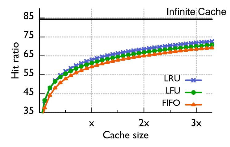
• Both LRU and LFU outperforms FIFO slightly
