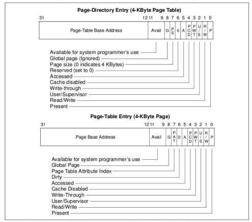
Figure 3-14. Format of Page-Directory and Page-Table Entries for 4-KByte Pages and 32-Bit Physical Addresses
