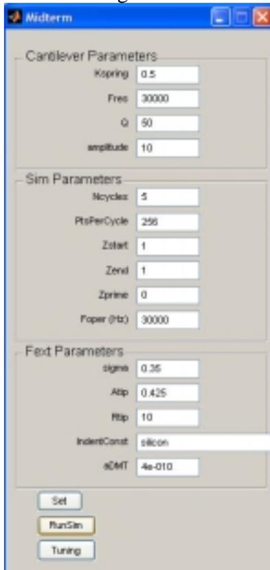
**Fres** – define your desired resonance frequency in Hz, the GUI will use this and Kspring to determine Mtip, etc.
