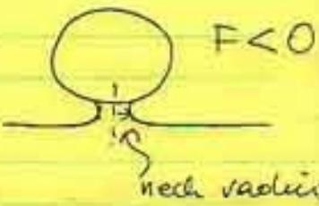
The force at which the neck breaks can be determined from the condition
