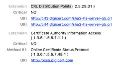
Figure 13.6: The CRL and OCSP fields in the certificate from Fig. 13.4.
