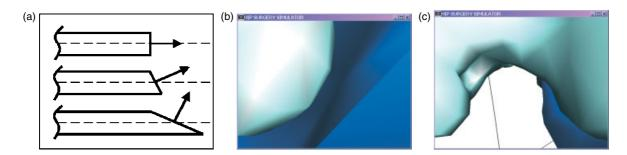
Figure 7. Comparison of arthroscopes with varying viewing angles. The camera angle describes the camera viewing direction; the angle is measured from the axial direction of the tool to the viewing direction. (a) Arthroscopes with  $0^{\circ}$  (top),  $30^{\circ}$  (centre) and  $70^{\circ}$  (bottom) viewing angles. (b) Computer-generated view from arthroscope with  $0^{\circ}$  viewing angle. (c) Computer-generated view from arthroscope with  $70^{\circ}$  viewing angle
