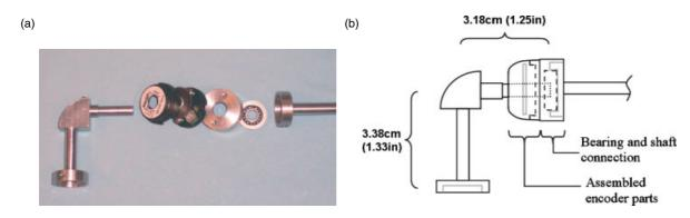
Figure 4. Encoder link components (a) and assembly. (b) Diagram of the assembled link
