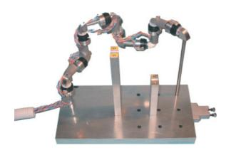
Figure 11. Encoder linkage with generic tool inserted in one of machined holes
