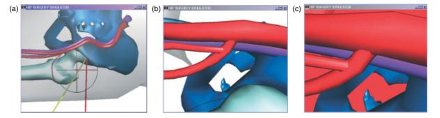
Figure 8. Proximity warning system. (a) Sphere representing safe area for tool operation. (b) Arthroscope view from within the safe sphere. (c) Arthroscope view from outside the safe sphere. As the arthroscope moves outside of the spherically-defined safe region and toward the femoral artery, the screen background changes to red to warn the surgeon
