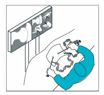
Figure 2. A computer-aided navigation system for arthroscopic hip surgery using a linkage tracking mechanism. Two encoder chains track the position of the surgeon's arthroscope and other tools. An additional screen in the operating room displays computer images of instruments and the patient anatomy from multiple views
