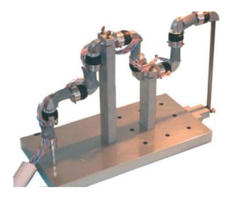
Figure 5. Tracking linkage locked in initialization configuration
