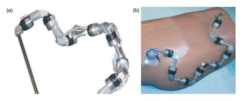
Figure 3. Encoder linkage for position tracking. (a) Tracking linkage prototype. (b) Linkage applied to a hip model. The linkage is redundant with extra degrees of freedom, to increase flexibility and ensure that the linkage remains out of the surgeon's work space
