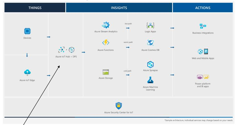
Uses MQTT or OASIS Advanced Message Queue Protocol (AMQP) DPS – Device Provisioning Service
