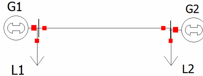
Fig. 6: Two bus system demonstration
