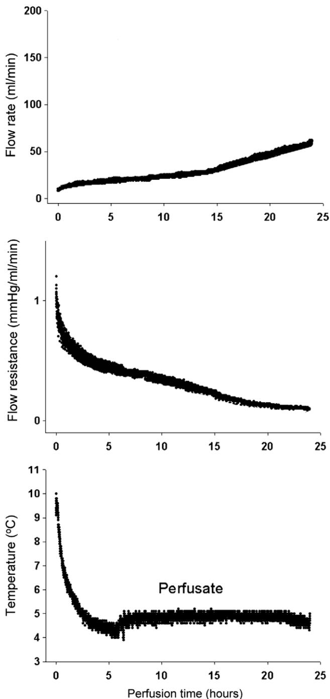
**Fig. 5.** Physical parameters (flow, resistance and perfusate temperature) measured on the LifePort<sup>®</sup> perfusion machine during 24 h hypothermic perfusion of a porcine pancreas. Pancreas weight = 87 g; the level of edema after 24 h = 139%, and the islet yield = 247,950 IE (islet equivalents; IE are determined using the universally accepted standard convention for quantifying islets, which inherently have a wide distribution of sizes ranging from <50 to >400  $\mu$ m diameter [134]).
