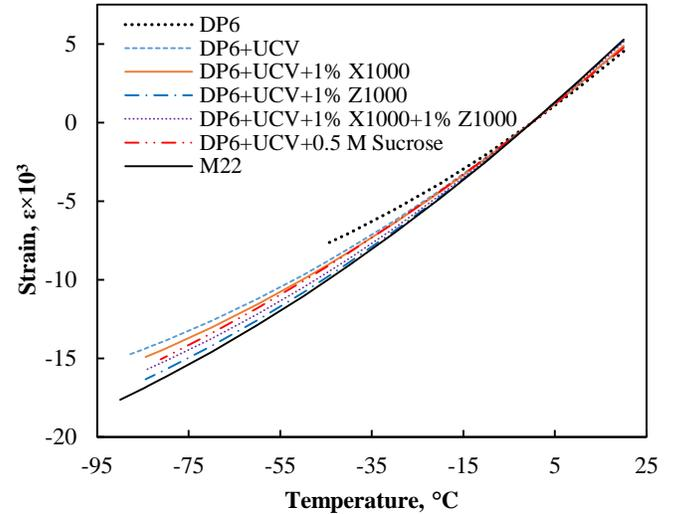
**Figure 1 Polynomial approximations of thermal Strain for all the materials used in the study.**
