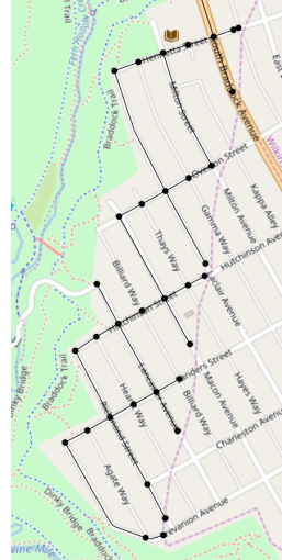
(b) The plowing graph is limited by an artificial district border on the right (dashed). The routing graph (not shown here) however expands beyond the border, thereby drastically reducing the number of U-turns needed if the streets would end at the district border.
