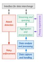
Figure 2: Components in an instance of a security monitor implementation
