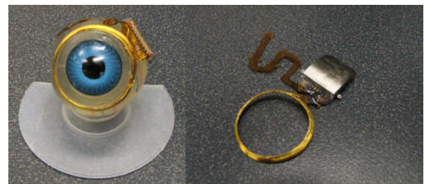
Fig. 2. Second-generation hermetically-packaged 16-channel Boston retinal prosthesis.
