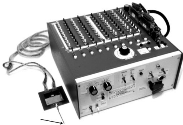
FIGURE 1. Electrical stimulation apparatus. Current sources are housed in the switch box. Each switch is connected by a multiwire cable to bonding pads on a printed circuit board (small, square structure, left), which was attached to the side of the patient's face during surgery. A microfabricated, polyimide ribbon cable connects the bonding pads to the stimulating electrodes, located at the distal end of the polyimide strip (arrow). Only the distal-most region of the polyimide strip containing the electrode array was inserted into the eye.
