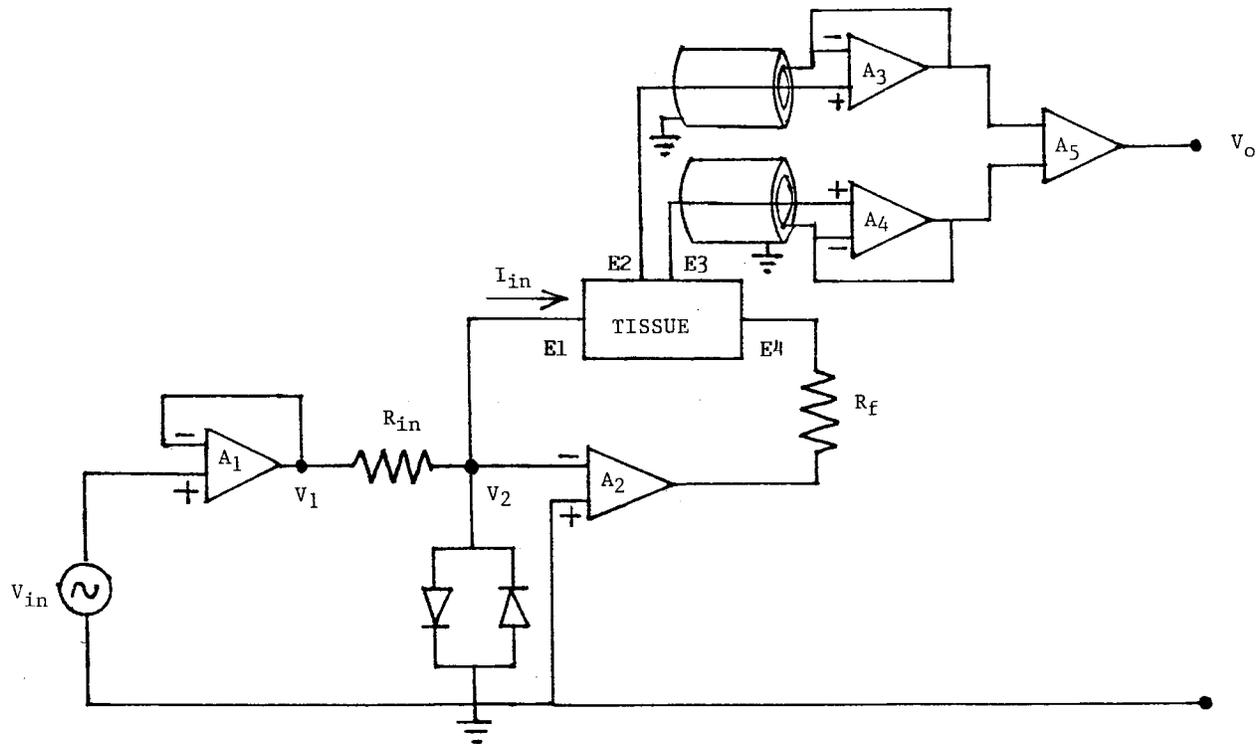
Fig. 2. The circuit for delivering current and measuring voltage across the conductivity cell. Constant current  $I_{in}$  is generated in the lower portion of the circuit and fed across outer electrodes  $E1$  and  $E4$  of the four electrode array. Inner electrodes  $E2$  and  $E3$  are used to measure the resulting voltage difference across the sample.
