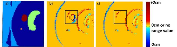
Fig. 8. (a) Image segmentation performed on the original image, (b) the depth map relative to the focal plane computed from light field captured by ASPs, and (c) the removal of inaccurate depths at the specular locations.
