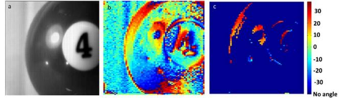
Fig. 7. (a) Scene with specular reflection, (b) the angle of polarization when no thresholding is performed, and (c) specular highlights tagged with a threshold of 40 mV.
