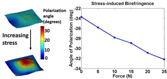
Fig. 5. Measuring change in polarization angle as a function of applied stress to polyethylene material. Minimum detectable force is 0.5 N.
