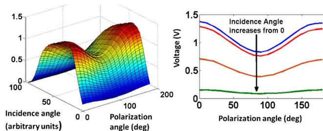
Fig. 2. Left figure plots common mode pixel output of polarization angle versus incidence angle in one-dimensional to show response  $\cos(2(\psi - \gamma)) * e^{-\theta^2}$ . Right plot shows cross section of this response at different incident angles.
