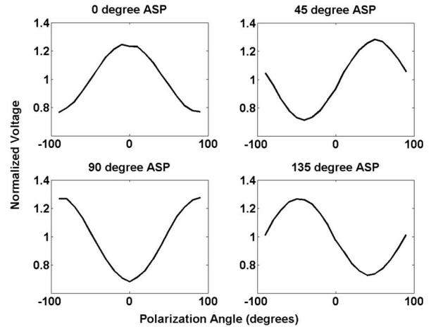
Fig. 3. Polarization response for ASPs with grating orientations of 0, 45, 90, and 135 degrees. Extinction ratios of approximately 2 were recorded.
