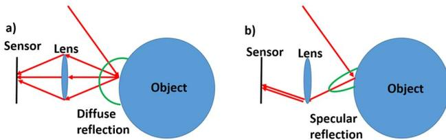
Fig. 6. (a) Diffuse reflection versus (b) specular reflection. Notice how the image sensor only receives rays from one specific angle in specular reflection which violates the Lambertian assumptions often made in computer vision algorithms.
