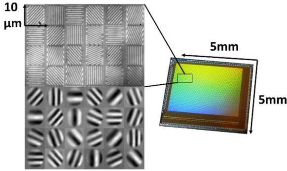
Fig. 1. Angle sensitive pixel (ASP) image sensor fabricated in 180 nm CMOS composed of 6 × 4 tile. The lower figure shows the corresponding two-dimensional angular point spread responses.
