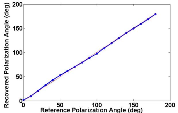
Fig. 4. Recovered polarization angle versus reference angle. The average deviation was around 1.12 degrees.
