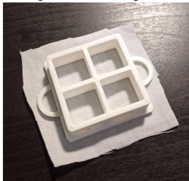
Figure 11. Measuring filter material
