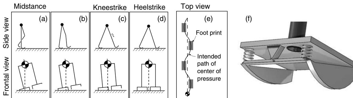
Fig. 5. (a-d) Side-to-side lean as guided by foot shaping. (e) Schematic of intended center of pressure path as a result of the side-to-side lean. (f) Schematic of the soft heel (left foot). The pivoting springs are at the heel. The asymmetric rubber-coated rails couple sideways lean to foot roll. The pivot and springs eliminate indeterminacies at the simultaneous impact of the two foot rails while maintaining stiffness against yaw and in the up-and-down direction.
