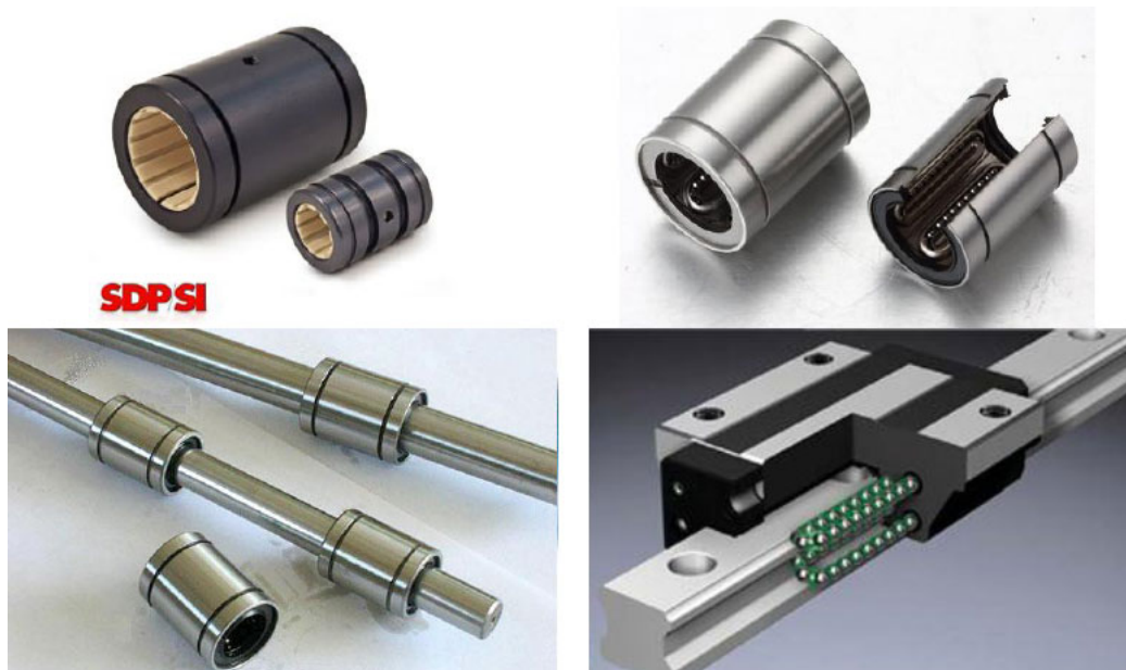
Linear bearings and rails. Top left: linear plain bearings. Top right: round linear bearing with recirculating balls. Bottom left: round linear bearings on rails. Bottom right: rectangular linear bearing on a multi-featured rotation-resisting rail.
