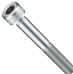
An 8-32 stainless steel socket cap screw with a hex drive and partial threads.
