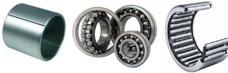
Left to right: Plain bearing (or bushing), ball bearings, and needle roller bearing.
