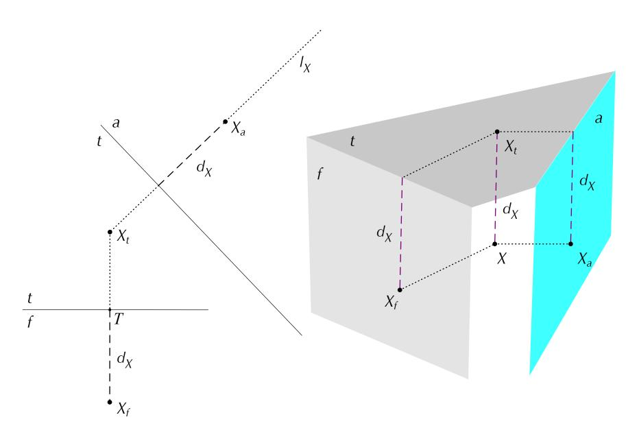
constructing an auxiliary view - transfer distance
