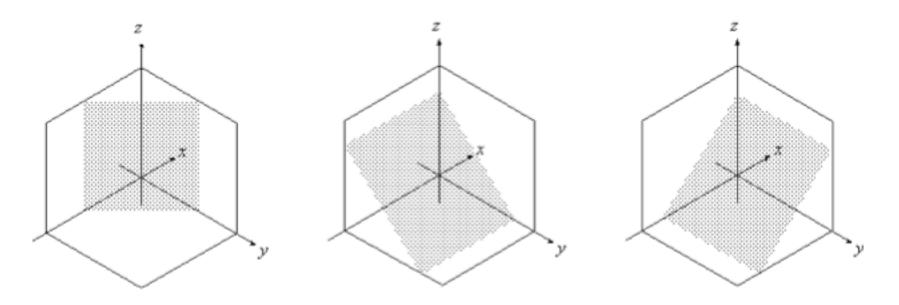
Given two adjacent views, a view using a picture plane perpendicular to the picture plane used in one or other view is an *auxiliary view*
