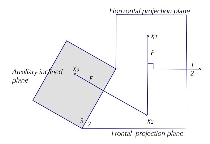
Given a point, X, in two adjacent views, t and f, construct an auxiliary view of X using a picture plane perpendicular to the picture plane of t.
