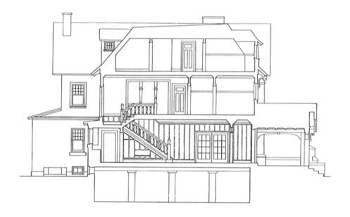
**ELEVATIONS** are developed with vertical picture planes that do not intersect the building
