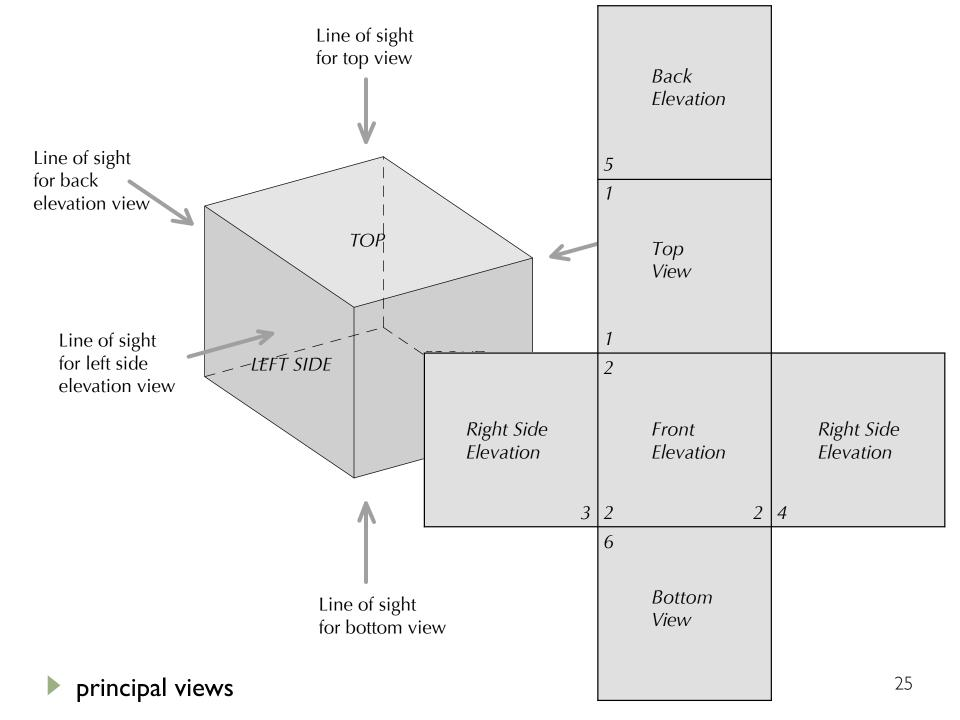
two orthographic views obtained from two perpendicular picture planes are called **ADJACENT**
