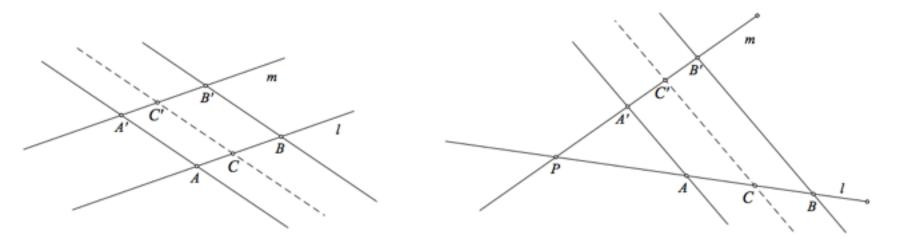
A'B' = AB ingles formed PA'/PA = PB'/PB intersection points are identical in measure parallel projections multiplies distances by a constant factor (could be 1)
