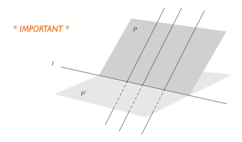
The image of a parallel projection in a plane onto another plane is the line common to both planes
