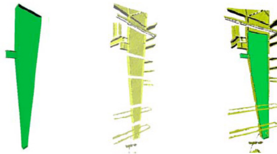
Figure 6: Example of the recognition progress for a steel column from case study B (Step 1: As-design model, Step 2: Range data from laser scanner, Step 3: Column recognized from Steps 1 & 2)
