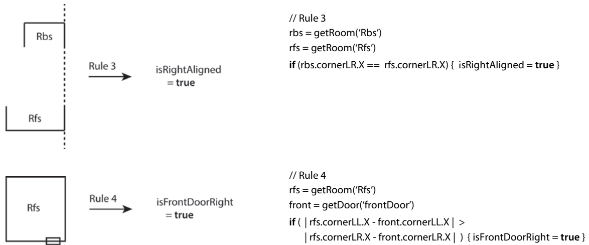
Figure 11 Right aligning rowhouse blocks: rules 3 and 4
