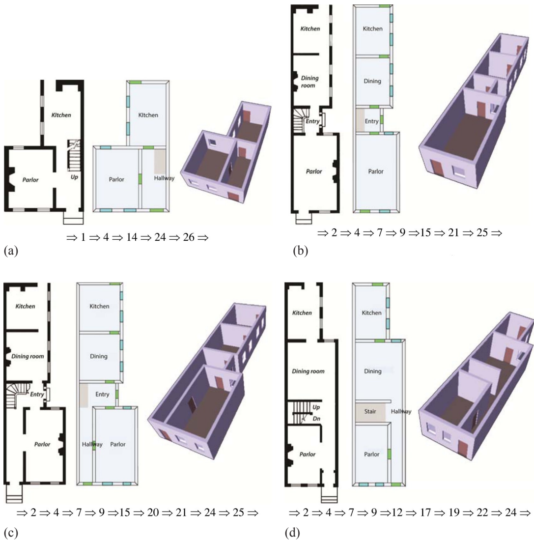
Figure 22. [In color online.] Layout results for the Baltimore rowhouse: (a) 3 East Montgomery Street, (b) 208 East Montgomery Street, (c) 236 East Montgomery Street, (d) 1029 South Hanover Street (shown in order of ground truth, generated layout, and feature input).
