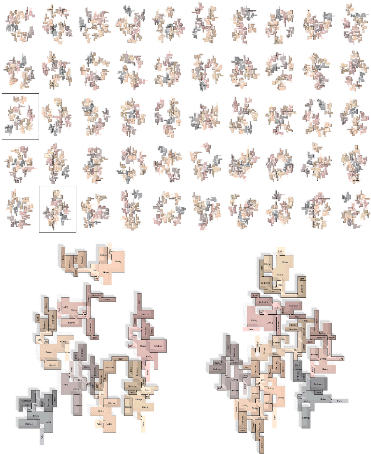
Fig. 22. 50 configurations produced by policy Adjacency, Area, Not Folding (5), and Daylight (50%) after 2000 steps. The configurations highlighted were selected for a more detailed description at the bottom.
