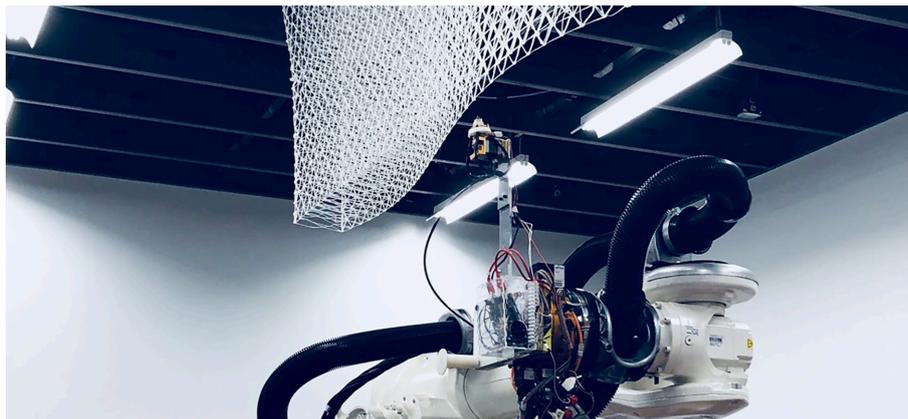
Figure 1. Free-Oriented Additive Manufacturing printing in the + $Z$  direction.
