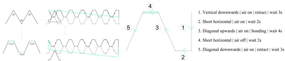
Figure 6. Physical constraint feedback into design process.
