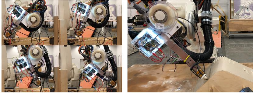
Figure 3. (Left) Tool operating within a 80cm space between vertical walls. (Right) FOAM applied over a non-planar surface.
