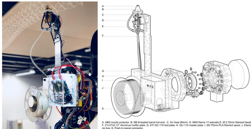
Figure 2. FOAM tool components: (Left) The working tool mounted on the robot arm. (Right) An annotated view of the components .
