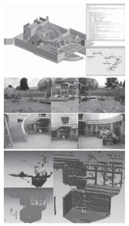
Figure 3. Case study (iv) examples; as-designed model, site condition, and as-built model.
