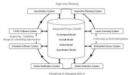
Figure 1. System integration diagram of ASDMCon project.
