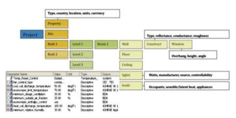
Fig. 4 Design elements for energy analysis not typically found in any design model
