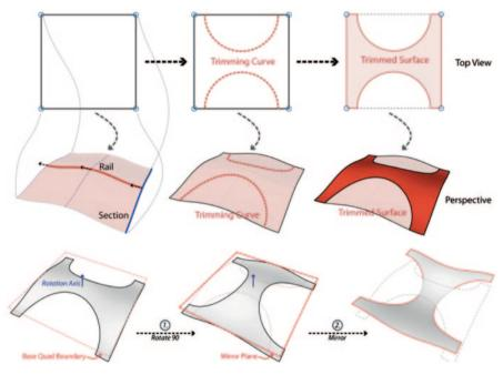
Fig. 13 Creating a trimmed surface for pattern ED\_03
