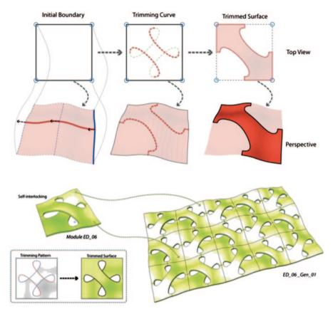
Fig. 16 Constructing the self-interlocking interwoven pattern ED\_06
