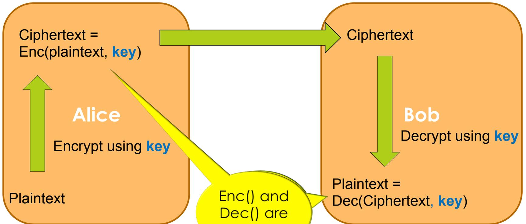
Alice uses the shared **key** to encrypt the plaintext to produce the ciphertext
