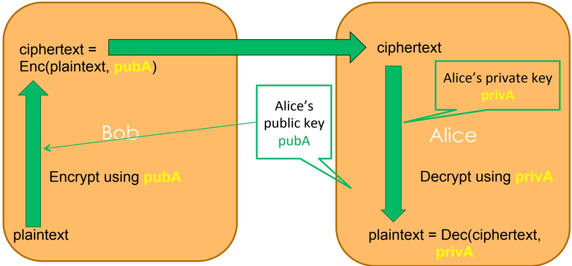
Bob uses Alice's public key to encrypt the plaintext to produce the ciphertext
