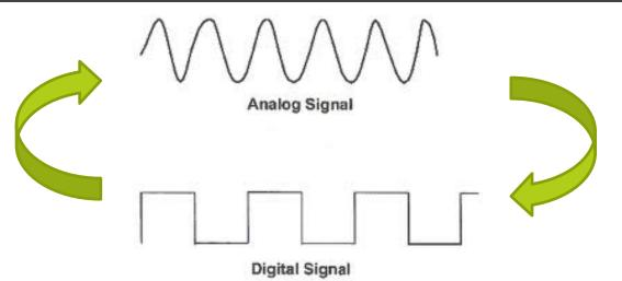
Modem (modulator - demodulator) transforms between physical states (analog) and bits (digital)
