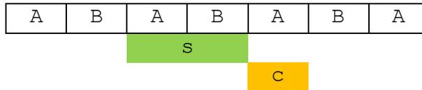
Output AB (256) in 12-bit, enter "ABA" with value 258 into the table
