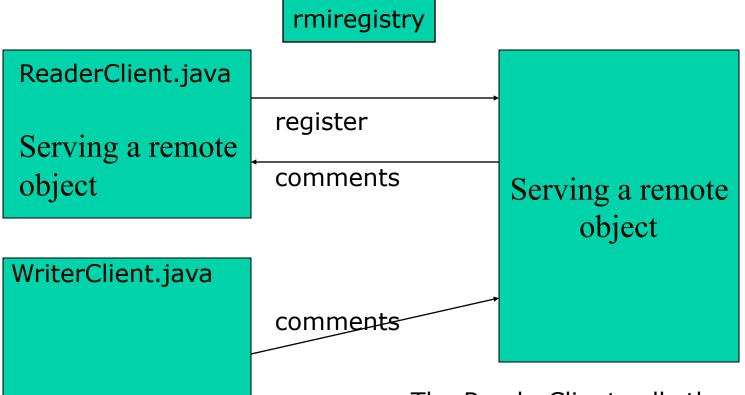
The ReaderClient calls the register method on the server side remote object. It passes a remote object reference.
